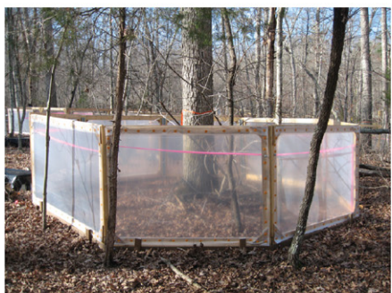
Forced air chamber warming experiment at Duke Forest, Hillsborough, North Carolina, USA (exp10, Pelini et al. , 2011). Photo credit: A. Ellison.
