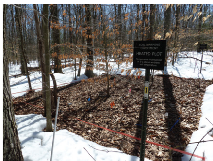
Soil cable warming experiment at Harvard Forest, Petersham, Massachusetts, USA (Melillo et al. 2017). Photo credit: A. Barker-Plotkin.
